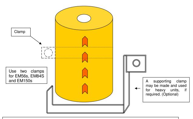
All units from EM21 to EM150s must be installed vertically with fuel inlet side at the bottom to avoid air lock.
