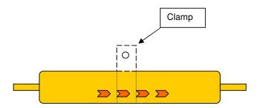
All units form EM4 to EM14 must be installed horizontally in petrol or diesel engines.
